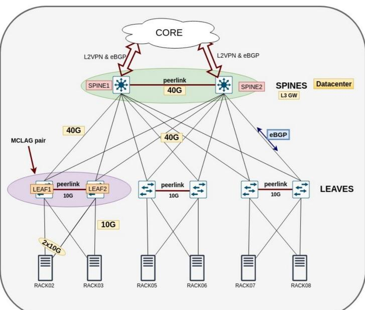
'All active links and switches' setup for redundancy.
